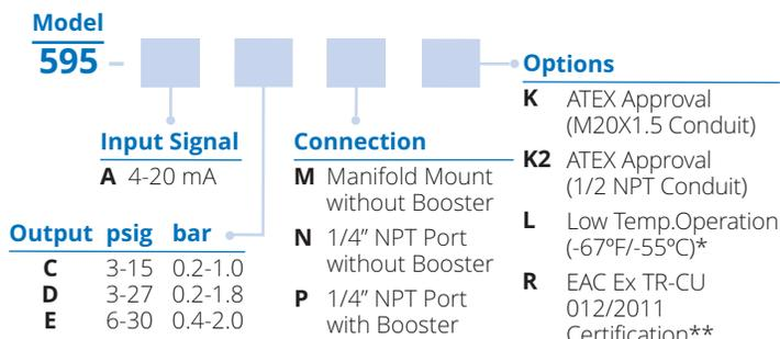
\* ATEX Exd, FM/CSA Explosionproof, EAC EX -40°F to 158°F (-40°C to 70°C) operation only
