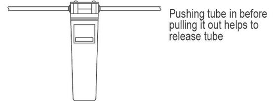
Pushing tube in before pulling it out helps to release tube
