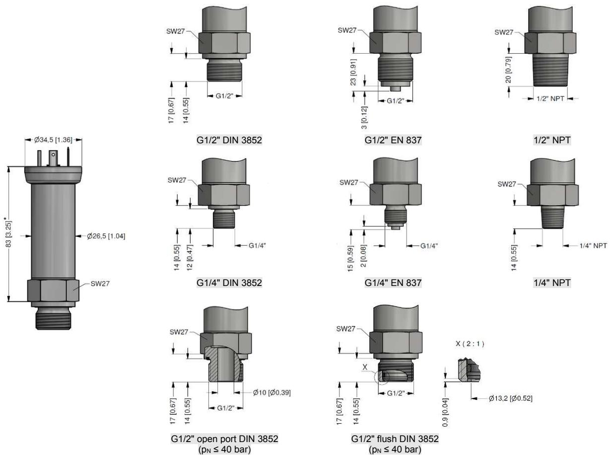
\* total lengths increase by 9 mm for  $p_N \geq 100$  bar with the optional accuracy  $\leq \pm 0.25$  % FSO
